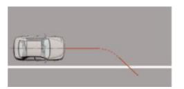
8.3.3.1.3. The subject vehicle speed during the test up to the point of system intervention shall be 72 km/h +/- 1 km/h.
