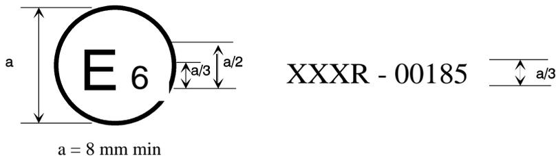
The above approval mark affixed to a vehicle shows that the vehicle type concerned has been approved in Belgium (E6) with regard to Direct Vision pursuant to UN Regulation No. [XXX]. The first two digits of the approval number indicate that the approval was granted in accordance with the requirements of UN Regulation No. XXX in its original form.
