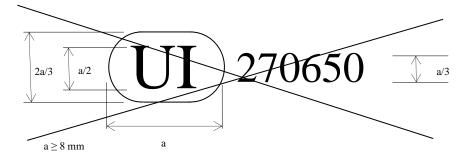
The above Unique Identifier shows that the type concerned has been approved and that the relevant information on that type approval can be accessed on the UN secure internet database by using 270650 as Unique Identifier. Any leading zeroes in the Unique Identifier may be omitted in the approval marking."
