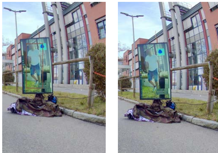
Figure 21: Result discrepancy due to changing lighting conditions due to cloudiness and changing position of the sun.
