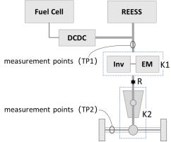
Note: measurement point for TP2 represents both axle shafts.
